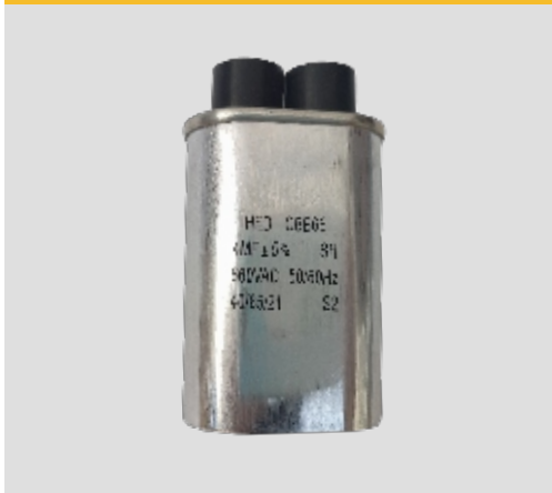
4 Mf capacitor, Lester charger
